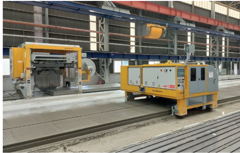
Automatic Plotter and multi-angle saw working fully automatically
