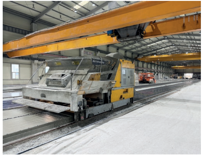
2.4m double panel EVO2 Extruder machine during casting
