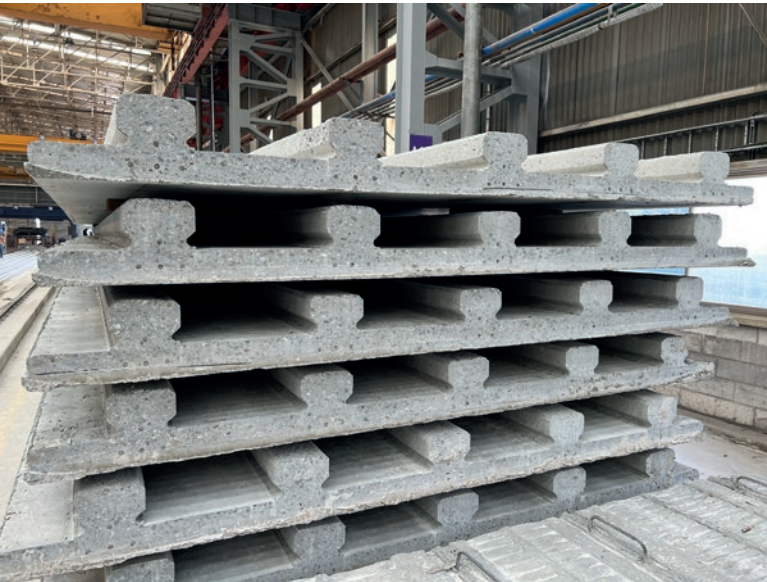
Half slab and hollow core slabs produced with the locally manufactured Slipformer
