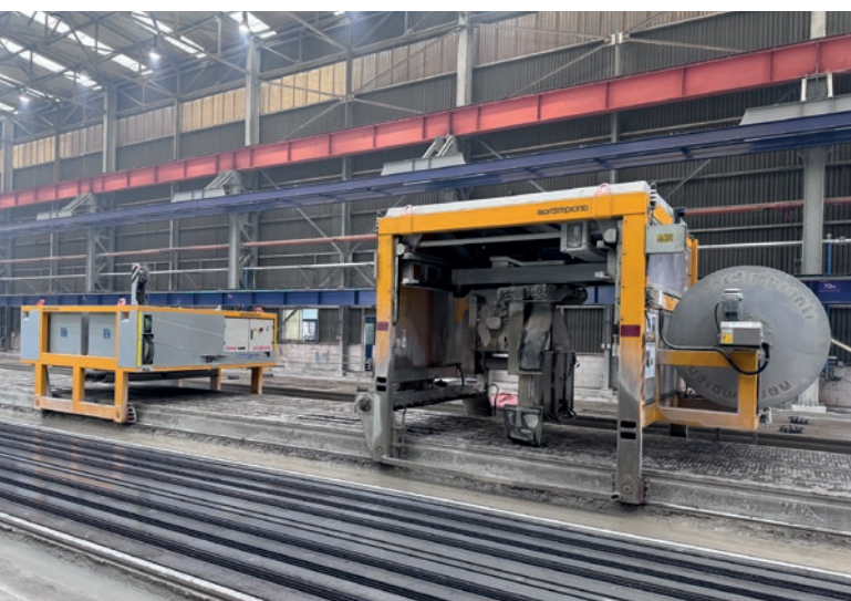
Automatic multi-angle cutting saw with counterweight trolley
